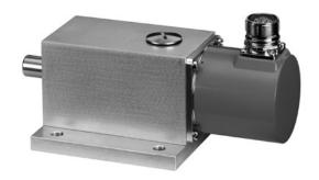
In applications where the encoder is driven by use of gears, chains, belts etc. and the permitted axial and radial shaft loads are exceeded, we recommend the use of the special designed bearing box which has stronger bearings.
