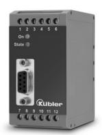
This compact signal converter with pulse inputs for two incremental encoders or measuring systems allows converting a frequency as well as sum, a difference, a product or a ratio between two frequencies into an analog signal. The integrated RS232 interface transmits the result of the connected inputs in the form of a serial signal.
