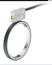
Thanks to its installation depth of min. 10 mm, the bearingless magnetic rotary encoder RLI200, comprising a magnetic ring and sensor head, is ideally suited for plants and machinery where space is very tight. The non-contact measuring principle allows for error-free use even under harsh environmental conditions, as well as ensuring a long service life.
