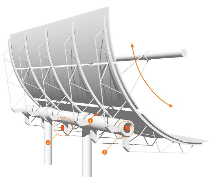
A parabolic mirror concentrates the sun's energy, thanks to its curved surface, onto a receiver pipe running along the inside of the curved surface.
