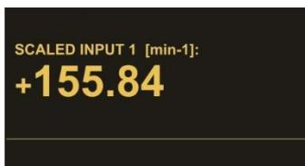
In this display, the respective input frequency of sensor1 is converted according to its adjusted parameters („OPU-Menu” in safety device) and shown in the display. \*) See chapter [0](#)
