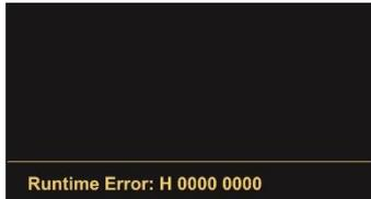
Error messages from the safety device are indicated as a hexadecimal number (H) given in the status line of the display. A listing of all available numbers and the associated errors can be found in the manual of the safety device.
