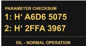
This display shows the CRC checksum of the stored parameter values in the safety device.
