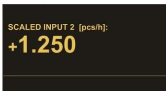
In this display, the respective input frequency of sensor2 is converted according to its adjusted parameters („OPU-Menu” in safety device) and shown in the display. \*) See chapter [0](#)
