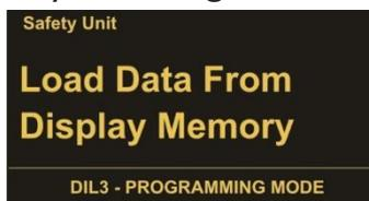
To load the parameters for a safety device from the flash memory of the SMCB.1, select "Load Data from Display Memory" and confirm with OK.
