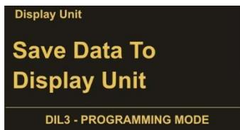
To save parameters in the SMCB.1, please select „Save Data To Display Unit“ and press OK to confirm.
