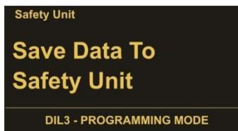
Select „Save Data To Safety Unit“ to save the respective parameters in that unit. Then press OK to confirm.
