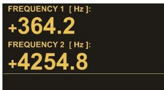
Both input frequencies of sensor1 and sensor2 are indicated with one decimal place (see “Operational Mode” of the safety unit).
