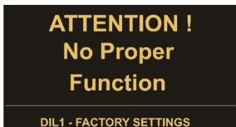
This mode is used to reset the safety unit back to its default values with the next power-up. No data entry at the SMCB.1 is possible here!
