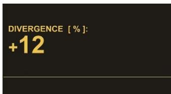
Indicates the divergence of both input frequencies in percent (see “Div. Calculation” of the safety unit).
