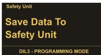
To save the parameter set in the safety device, select "Save Data To Safety Unit" and confirm with OK.
