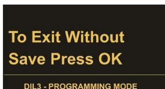
If the menu (after changing parameters) should be left without saving, the procedure „Exit Without Save Press OK“ must be confirmed with OK. Press button C to jump back to the storage menu.
