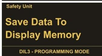
Select „Save Data To Flash Memory“ to save parameters of the safety unit into the flash memory of the SMCB.1. Then press OK to confirm.
