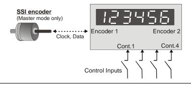
One SSI encoder only is connected to the unit.
