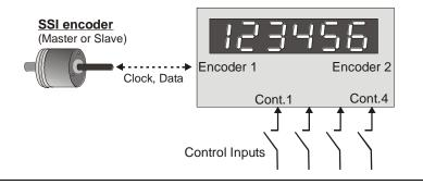
One SSI encoder only is connected to the unit.
