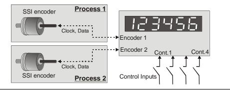
Both encoder inputs are connected to SSI encoders for individual evaluation. The encoders may have different resolutions and can operate at different Baud rates and individual scaling.
