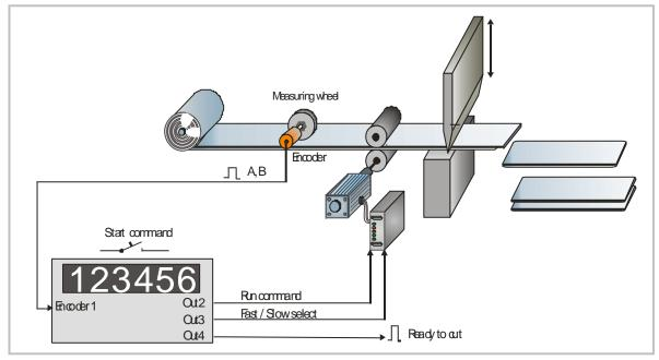
The Start command can be assigned to any of the front keys or to or to any of the Control Inputs, by attaching the RESET function to it (e.g. set parameter F06.052 to 1 to assign the Start function to the ENTER key etc.). Also an automatic reset function with a timed output signal can be used, in order to ensure automatic stepping of the cutting sequence without a remote start signal.
