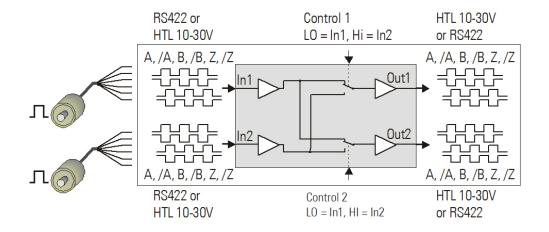
Both inputs can be individually set to either symmetric (differential) format using A, /A, B, /B, 0, /0 channels, or to asymmetric (single-ended) format using A, B, 0 channels only. Acceptable input levels are RS422, TTL and HTL 10 ... 30 V.
