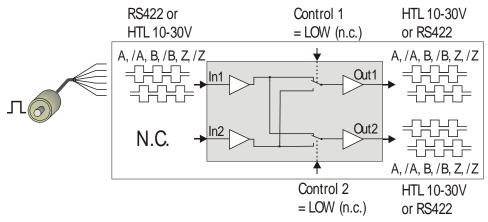
Input 1 is used as encoder input, and Input 2 remains unconnected. The input can be set to either symmetric (differential) format using A, /A, B, /B, 0, /0 channels, or to asymmetric (single-ended) format using A, B, 0 channels only. Acceptable input levels are RS422, TTL and HTL 10 ... 30 V.
