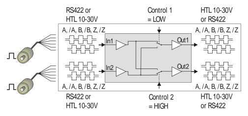
Both inputs can be individually set to either symmetric (differential) format using A, /A, B, /B, 0, /0 channels, or to asymmetric (single-ended) format using A, B, 0 channels only. Acceptable input levels are RS422, TTL and HTL 10 ... 30 V.
