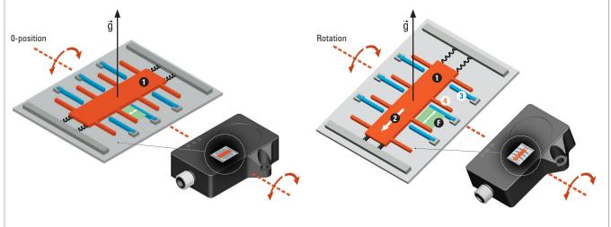
Intelligent sensor fusion of acceleration and rotation rate measurement for dynamic applications (types IN7x)
