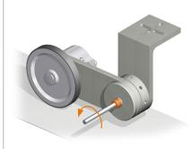
2. Turn the adjustment ring with a thin allen key or screwdriver until the desired preload is reached.
