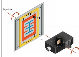
Intelligent sensor fusion of acceleration and rotation rate measurement Both measured values are combined in the inclinometers for dynamic applications. The effect is even faster and more accurate output results.
