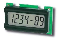
The timer module of the type 194 for PCB mount features a 6-digit LCD display and 2 voltage ranges (4.75  $\dots$  15 V DC and 9  $\dots$  60 V DC).
