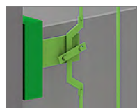
Mechanical trigger of the safety gear
