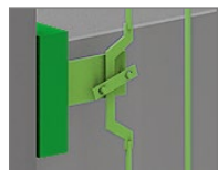
Mechanical trigger of the safety gear
