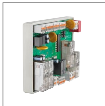
Kübler evaluation unit PSU02 (in the switch cabinet)
