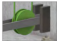
Tensioning device for overspeed governor
