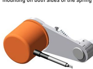
Mounting left (delivery state)
