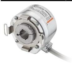
The optical Sendix F5883 multiturn encoder in the Motor-Line version stands out particularly because of its reduced overall depth of only 43 mm with a through hollow shaft up to 15 mm.
