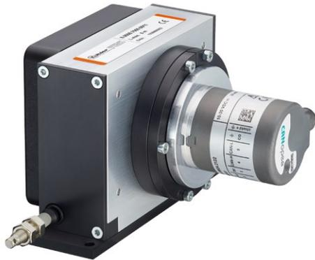
The draw-wire encoder C105 features a compact design. It is available with various wire types. All encoders with 58 mm synchro flange and 6 mm shaft, as well as analog sensors with redundant interfaces can be combined with this draw-wire mechanism. The cable and connector orientations of the encoder can easily be adapted to the position of the mechanism. A flexible wire outlet compensates mounting tolerances.
