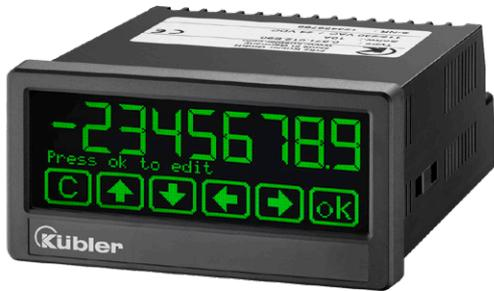
The process controller 573T with 2 analog inputs can be used in both single channel mode as well as in dual channel. In dual channel mode, all arithmetic operations are available for displaying the sum total, difference, ratio or the product. Inputs and outputs can be scaled separately.
