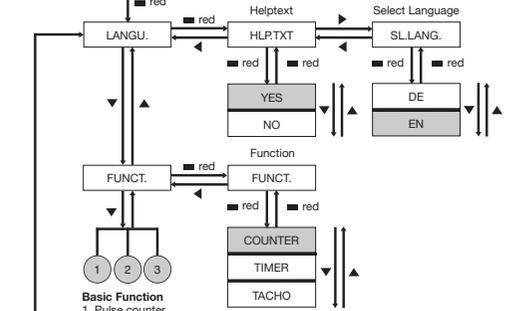
Changing the basic function causes all parameters to be reset to factory settings.
